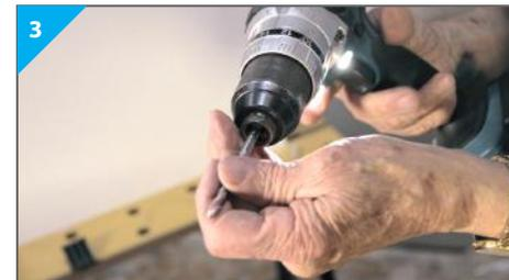
3 Secure a diamond core drill bit to your drill. Align the holes and start to drill carefully. Don't exceed 500rpm.
