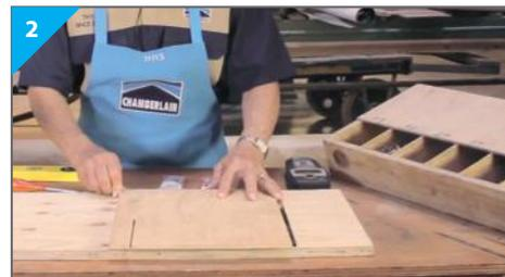
2 Place the wooden template on top of your mirror. Make sure all sides are perfectly aligned.
